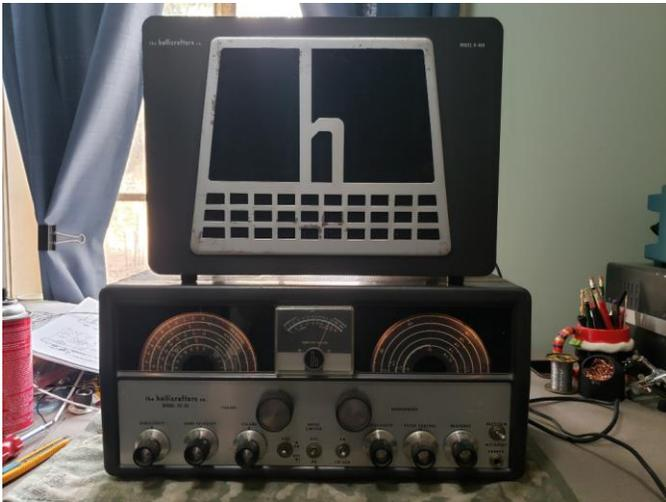
Then I did a full IF alignment of both the 50.5 KHz and 1650 KHz IF's. Then I did an RF alignment. The alignment itself took over 15 hours because I had to hunt down two failed components.
