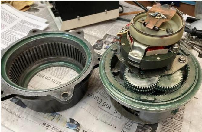
When you're all done, a rotator like this should be tested stop-to-top and then left in the North (centered) position. Put a label on it to remind the installer that it's all lined up for them. I also put on a service label with the date in case the rotator is stored for awhile.
