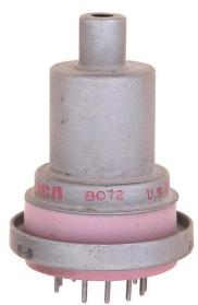
In 1971, Eimac upgraded the tubes to the 8072W etc. making them more rugged and rated them to withstand 50Gs.
