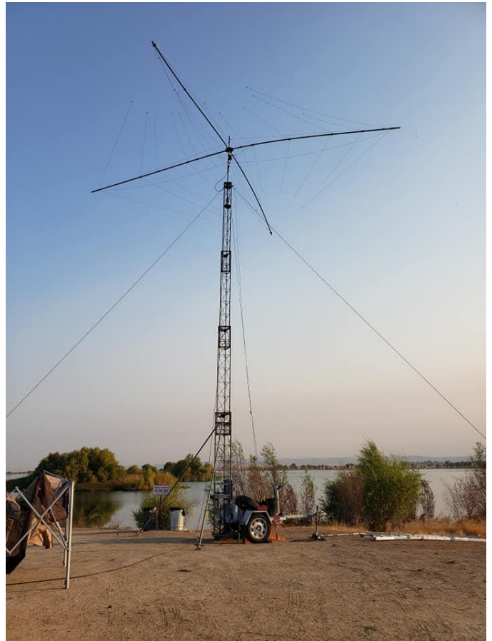
Tower trailer with Spiderbeam antenna.
