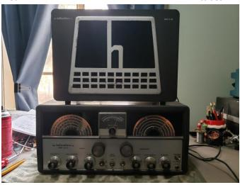
Then I did a full IF alignment of both the 50.5 KHz and 1650 KHz IF's. Then I did an RF alignment. The alignment itself took over 15 hours because I had to hunt down two failed components.
