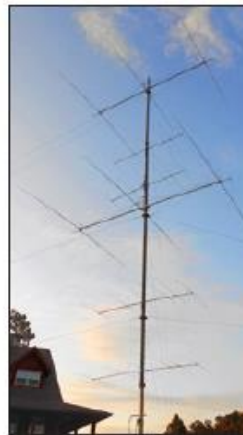
This is the 80 meter monopole. The top antenna is at 165 feet and the bottom one is at 80. The three-element Optibeam 80 meter Yagis were highly modified by Kurt Andersen, K7NV.
